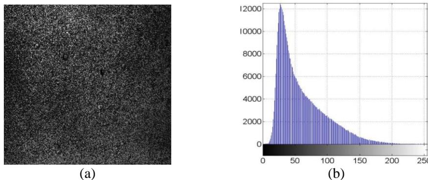
Figure 3. A typical speckle pattern and its histogram, applied on 5 hour age 40MPa concrete.
