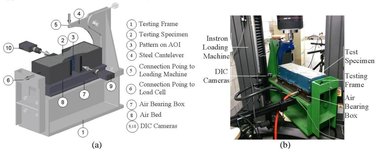
Figure 1. Schematic Illustration (a) and actual test setup (b) of Direct Tensile Apparatus
