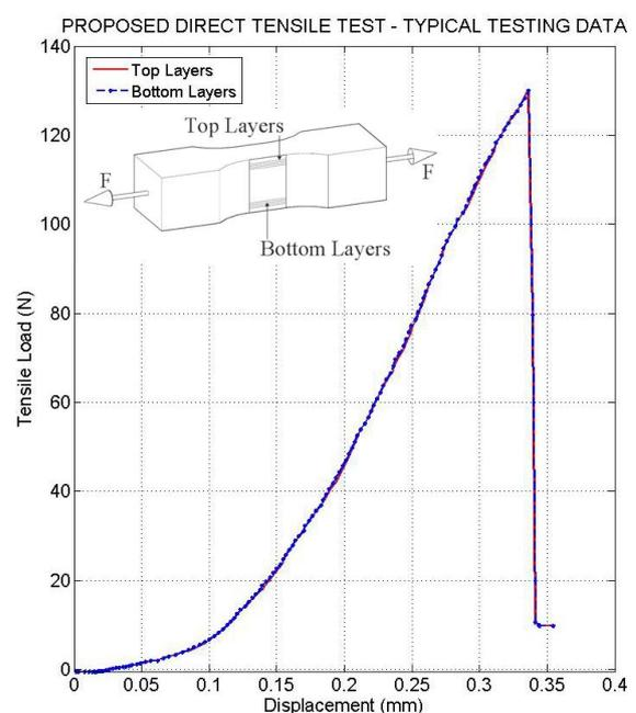
Figure 4. Load – Displacement of 40MPa concrete at 5-hour age.
