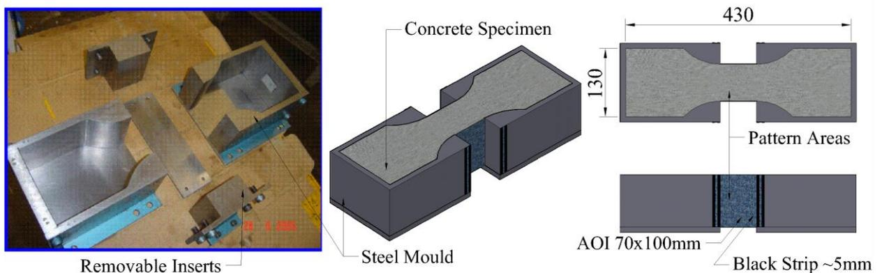
Figure 2. Testing Mould with Areas of Interest (AOIs)
