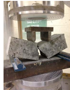
c) Flexure failure respectively
