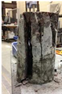
Figure 2.a) Columnar shear failure
