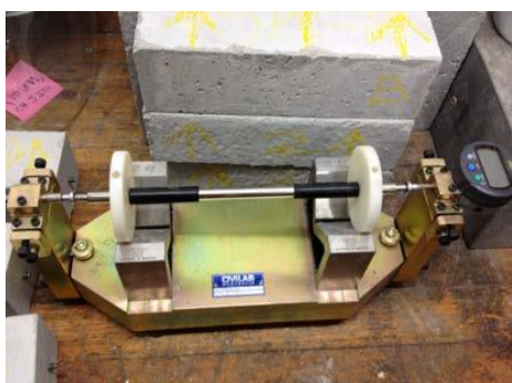
Figure 3a. Drying shrinkage test equipment 3b. Drying shrinkage results for LWSAC
