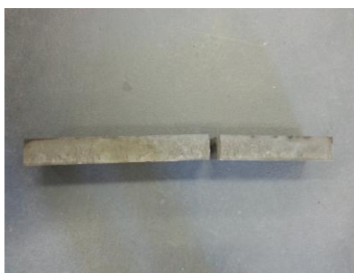
Figure 4a. Cracking pattern of specimens with BS05
