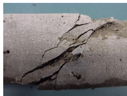
Figure 7b. Specimens cured for 182 days
