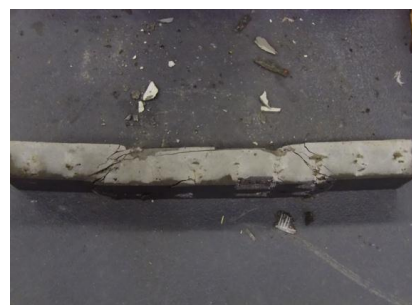
Figure 4b. Cracking pattern of specimens with BS50
