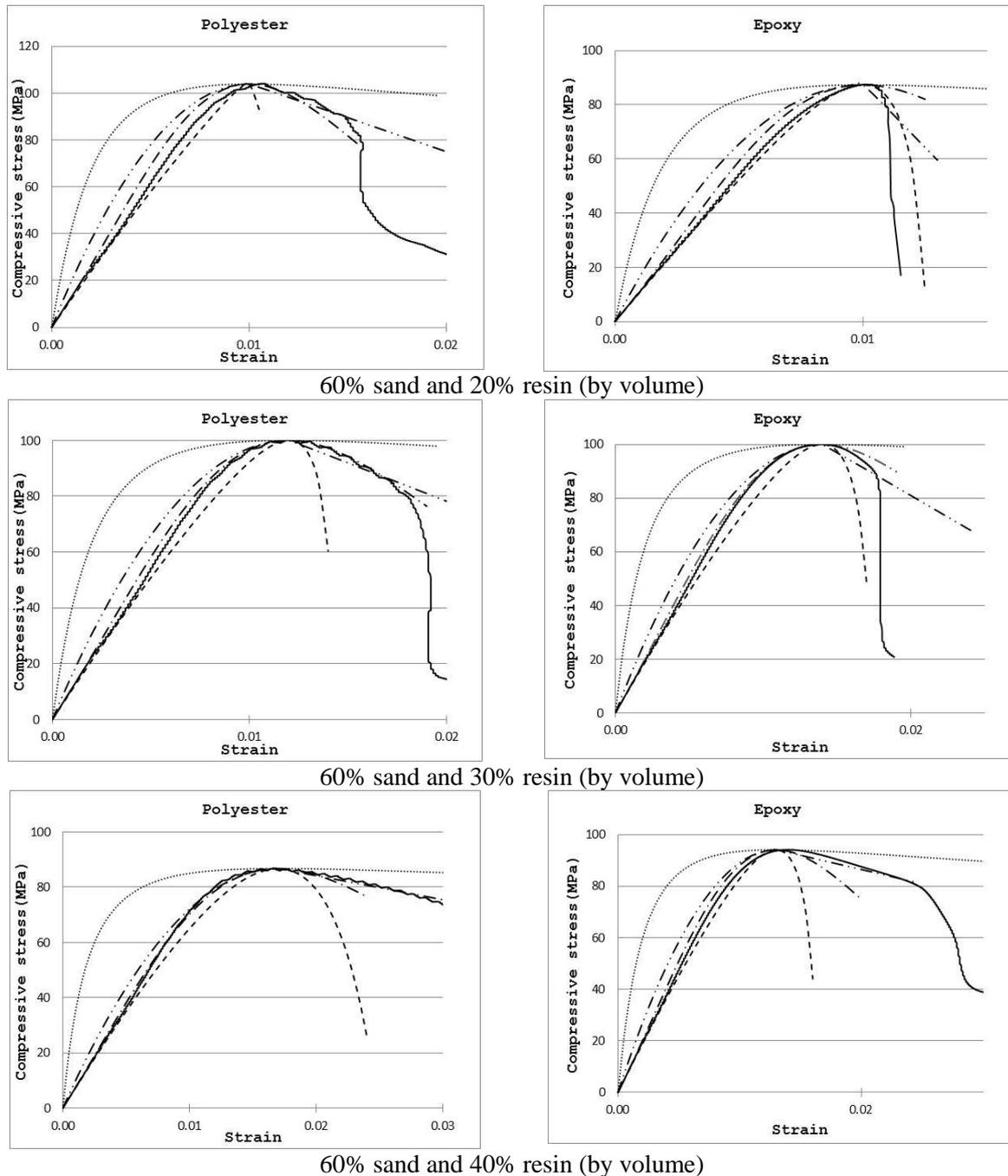
Figure 2. Experimental and predicted stress-strain relationships
