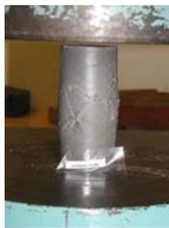
Figure 1. Compression testing
