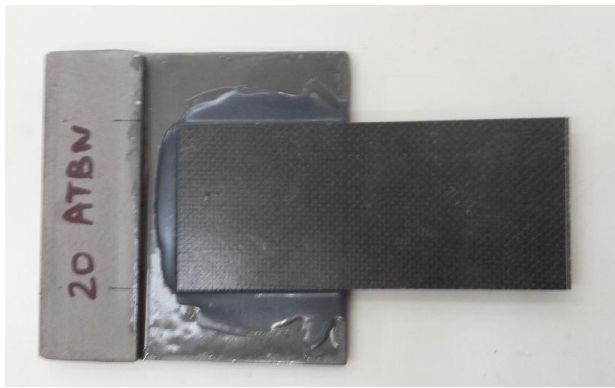
Figure 1. CFRP sheet bonded to the Steel plate
