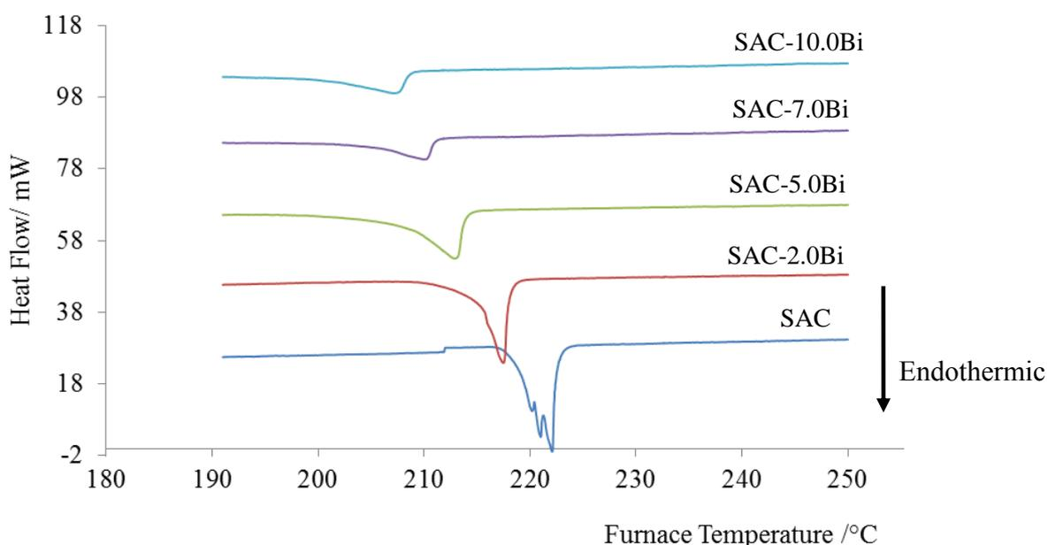
Figure 1. Effects of Bi substitution for Sn on the DSC thermogram of SAC alloy
