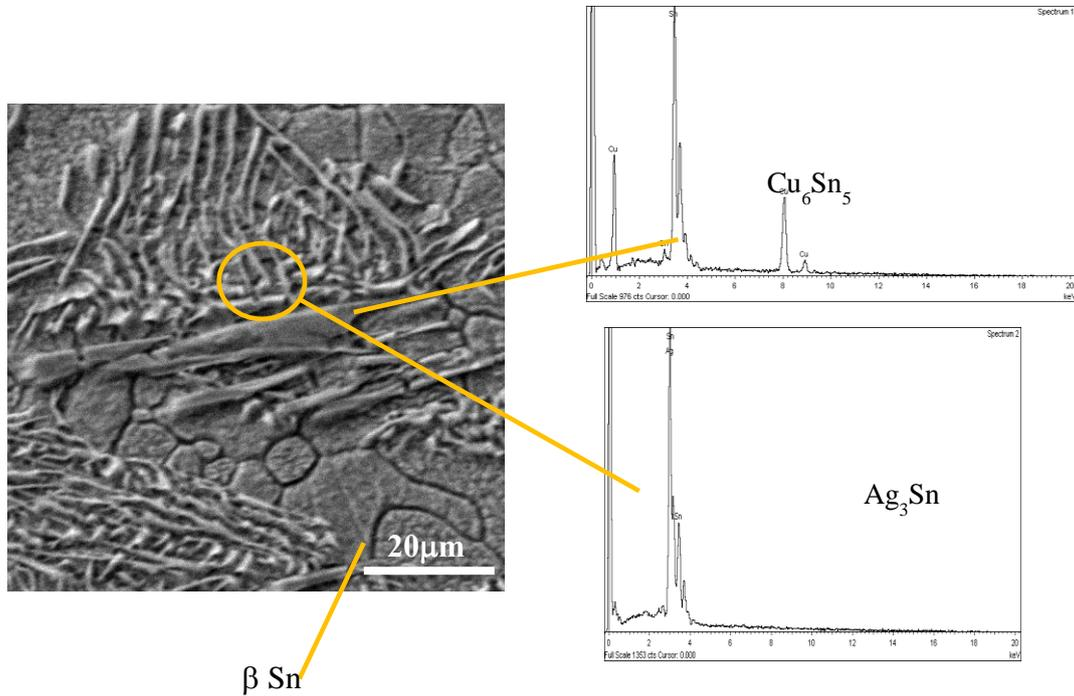
Figure 3. Typical microstructure in ingot alloy
