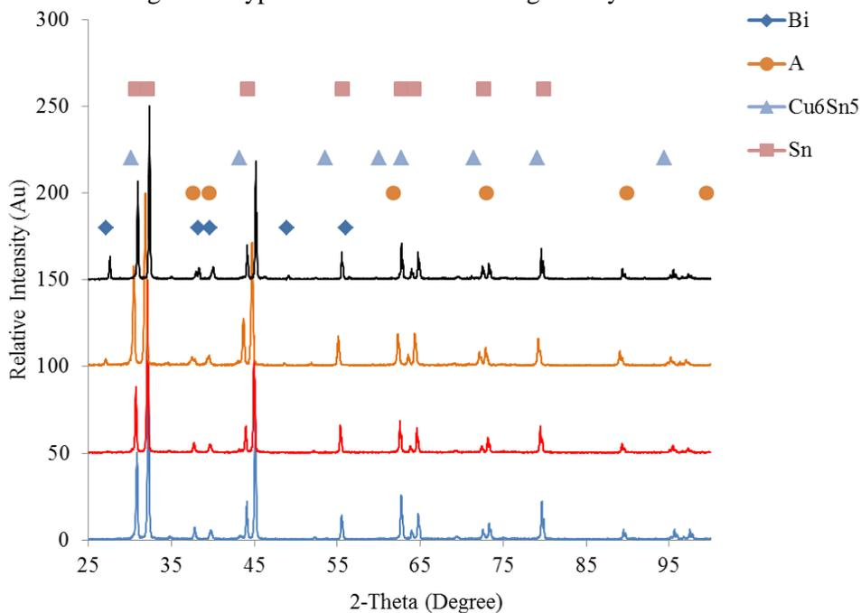
Figure 4. Effect of Bi substitution on appearance of Bi phase in ingot alloy
