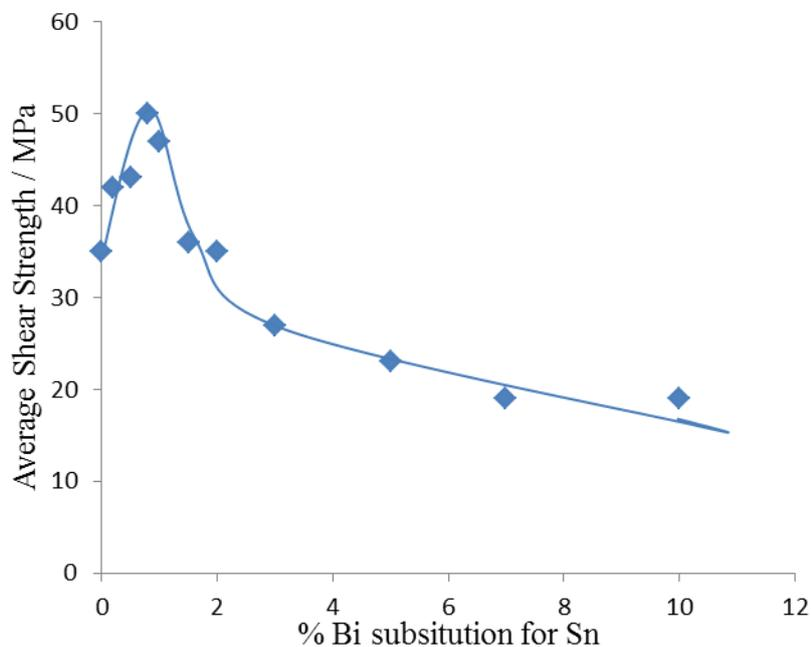
Figure 2. effect of Bi concentration on the shear strength of SAC-Bi alloys
