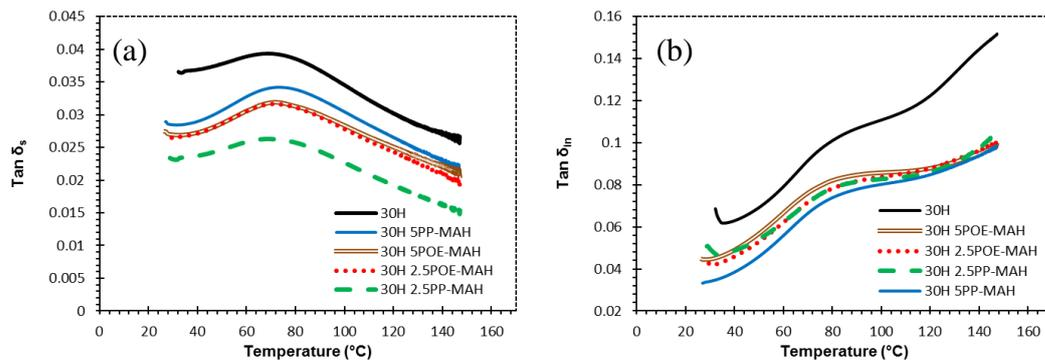
Figure 9. (a) System and (b) interphase damping ratio of coupled noil hemp fibre reinforced composites as function of temperature under DMA loading frequency of 1Hz
