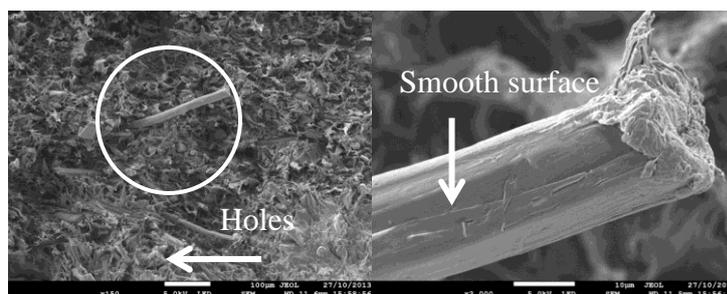
Figure 5. SEM micrographs of fractured surface for the 40 wt.% hemp fibre polypropylene composite with 5 wt.% MAPOE coupling agent
