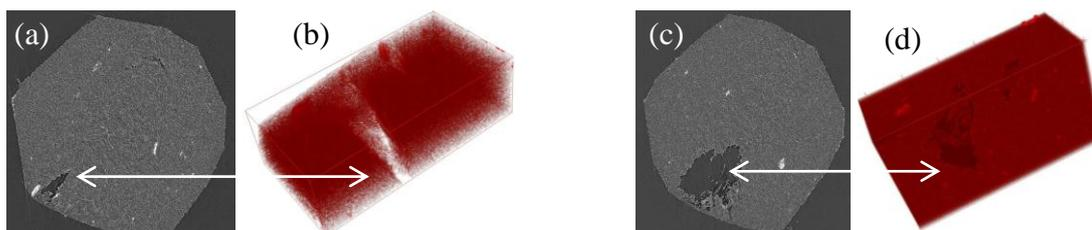
Figure 3. (a&c): Typical reconstructed x-ray microtomography images of the composite with 60wt.% hemp fibre which shows voids, (b&d): 3D views of associated voids in the composites
