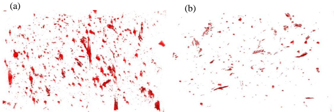
Figure 7. Noil hemp Fibre agglomerations in polypropylene matrix: (a) 40H and (b) 40H5MAPP
