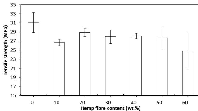
Figure 1. The influence of the fibre weight content on tensile strength of the noil hemp fibre reinforced polypropylene composites
