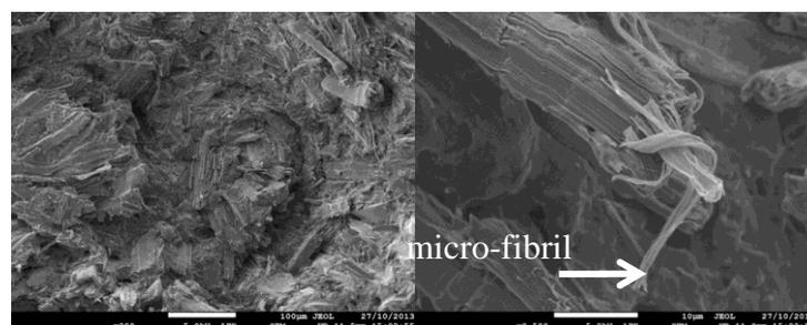
Figure 6. SEM micrographs of fractured surface for the 30 wt.% hemp fibre polypropylene composite with 2.5 wt.% MAPP coupling agent
