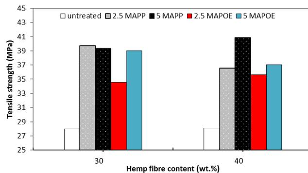
Figure 4. The influence of coupling agent type and their content on tensile strength of the noil hemp fibre reinforced polypropylene composites
