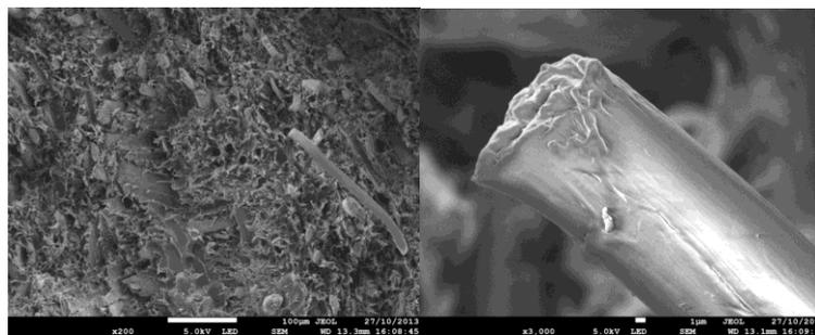
Figure 2. SEM micrographs of fractured surface for the 60 wt.% hemp fibre polypropylene composite without a coupling agent
