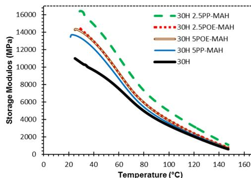
Figure 8. Influence of coupling agent addition on storage modulus values of of 30wt.%hemp sample
