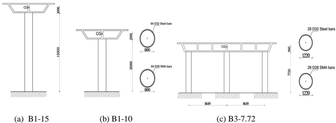
Figure 3. Prototype bridge bents studied
