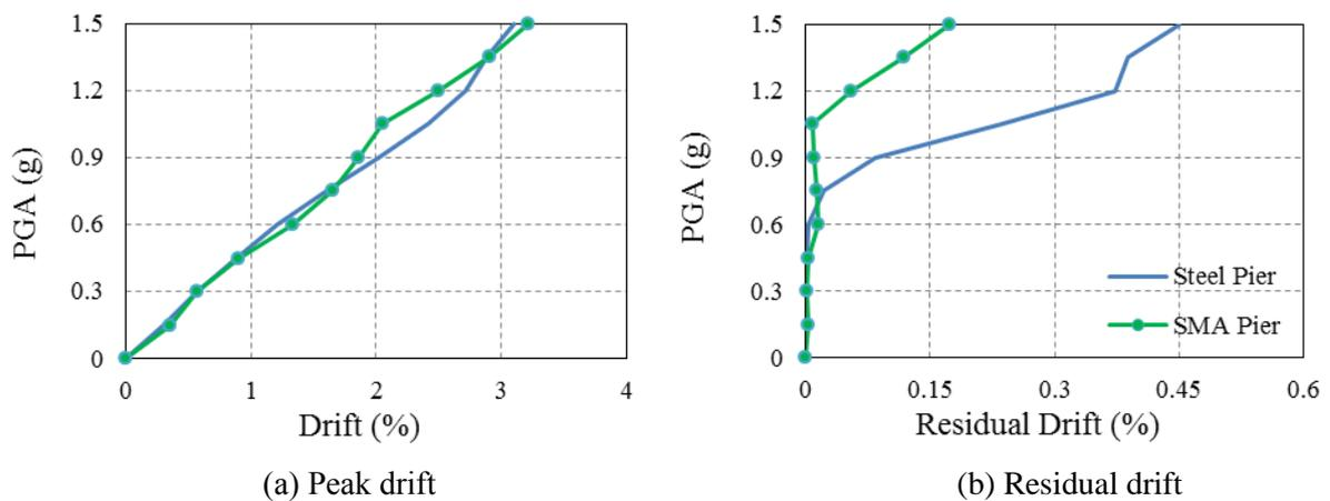
Figure 6. Response of bent B1-15 to Moorpark motion
