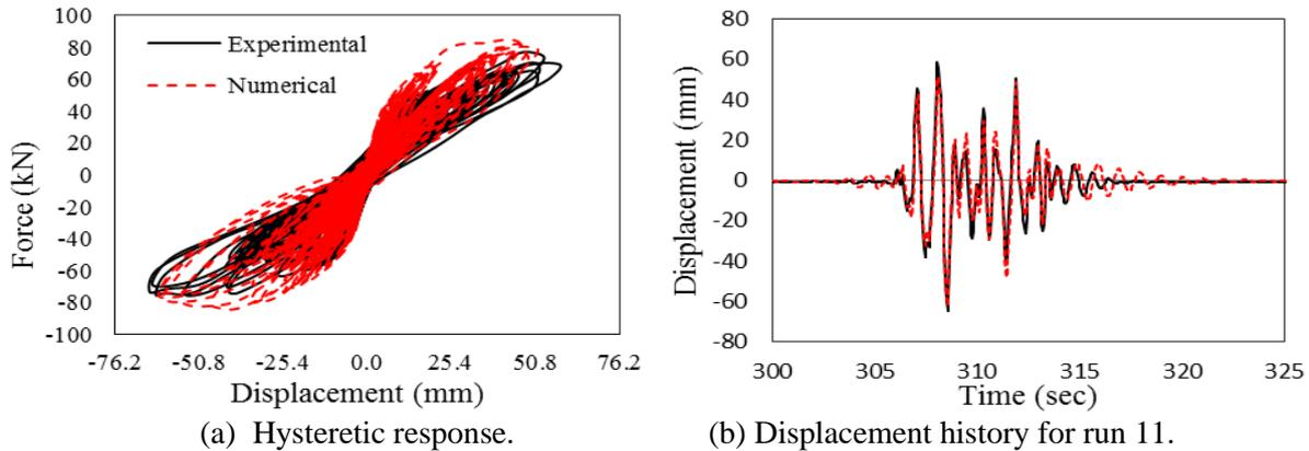
Figure 2. Response comparison: test result versus numerical result
