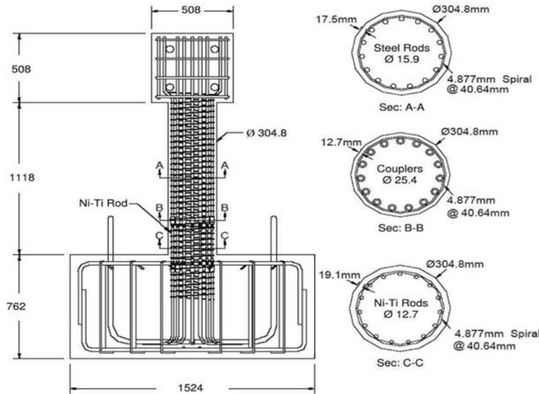
Figure 1. Details of SMA RC column (Saiidi and Wang, 2006)
