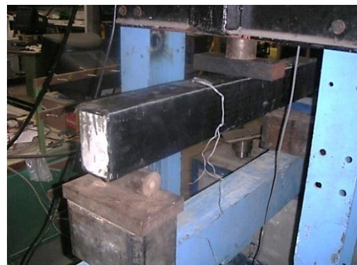
(a) FBD of Static Beams (b) Experimental Static Testing Figure 2. Static Testing of CFRP Strengthened Beam B1
