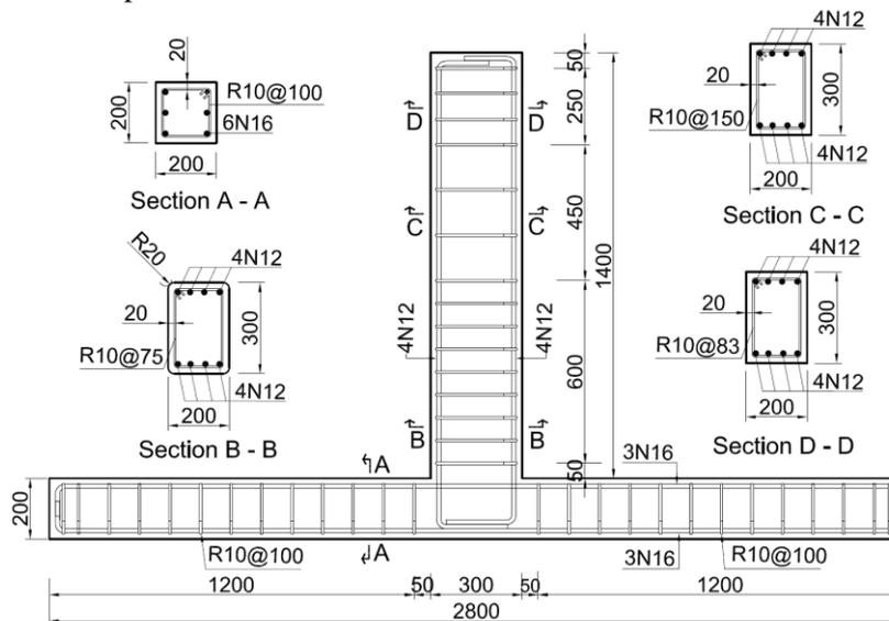
Figure 1. Reinforcement details of Specimens T0, TS, TS1 and TS2 (all dimensions in mm)
