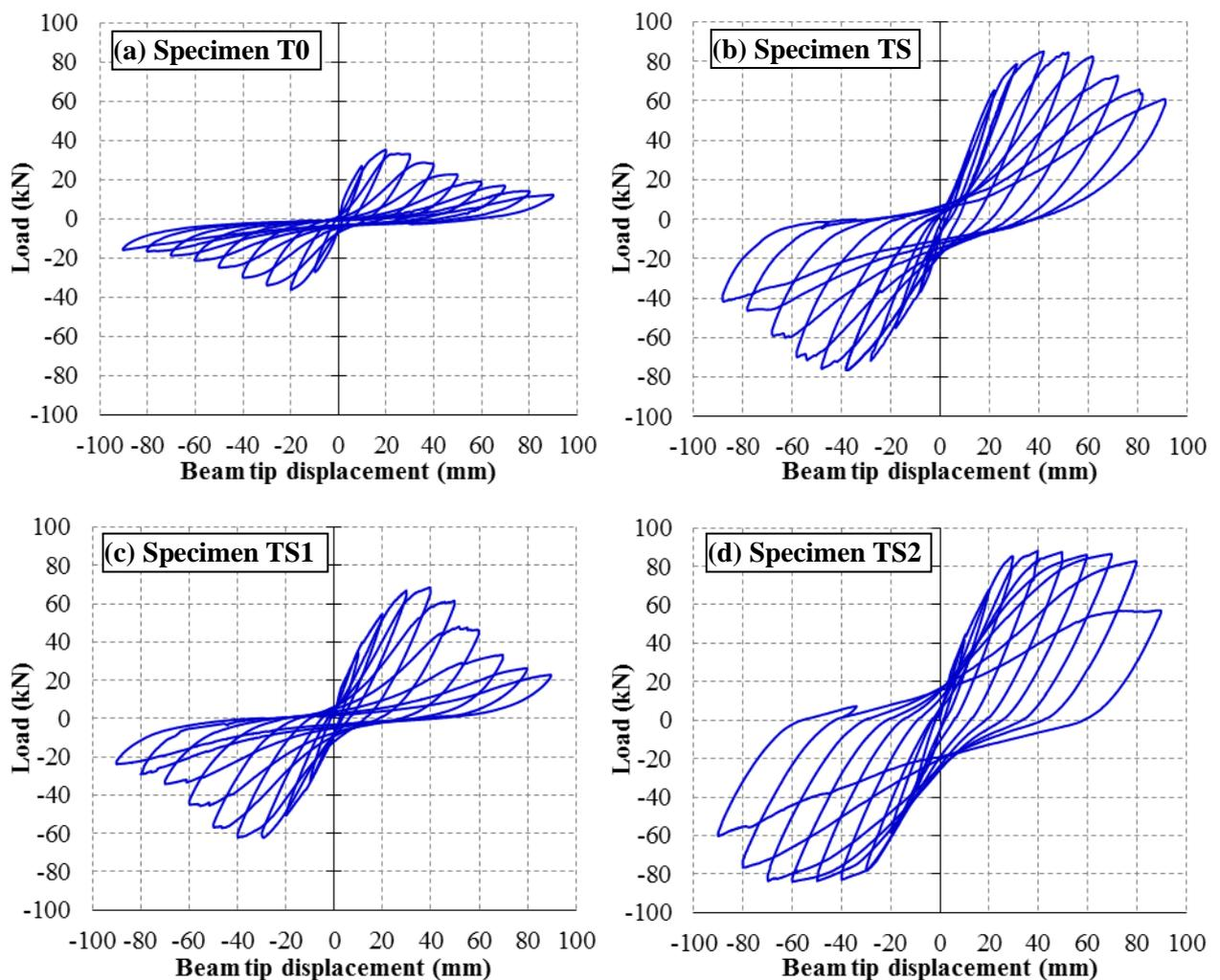
Figure 4. Load versus displacement response hysteresis of Specimens T0, TS, TS1 and TS2
