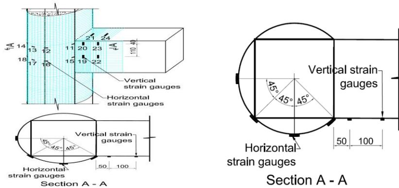
Figure 3. Position of strain gauges (all dimensions in mm)
