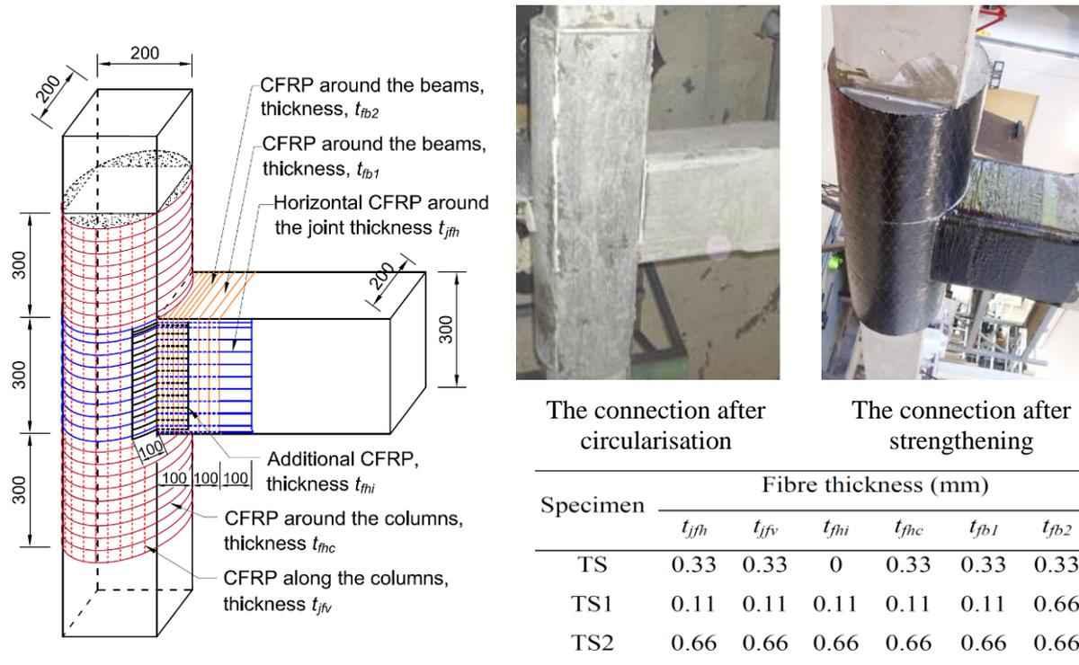
Schematic illustration of the strengthening of Specimens TS, TS1 and TS2
