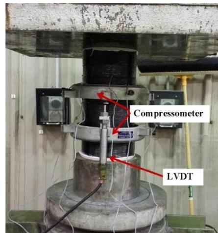
Figure 2. Compressometer
