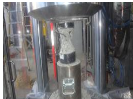
Figure 7. Confined concrete at failure
