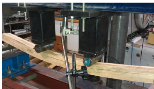
Figure 2. Four-point bending test setup for manufactured bamboo
