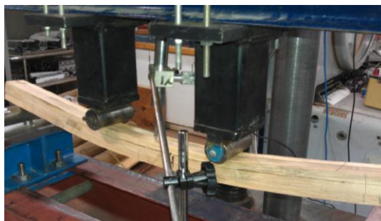
Figure 2. Four-point bending test setup for manufactured bamboo
