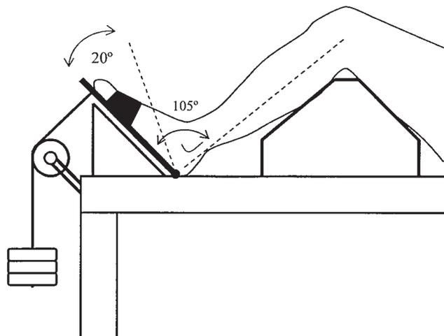
FIG. 2. A sketch of the custom-built testing device for dorsiflexion strength.
