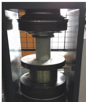
Figure 1. Uniaxial compressive test
