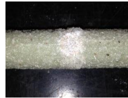
Figure 5. Crushing of the resin and fibre of GFRP bars (21 °C to 80 °C)
