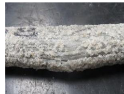
Figure 7. Interlaminar shear failure of the 12.7 mm and 15.9 mm GFRP bars (21 °C to 80 °C)
