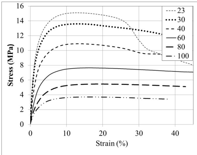
Figure 2. Typical stress-strain behaviour at different temperature
