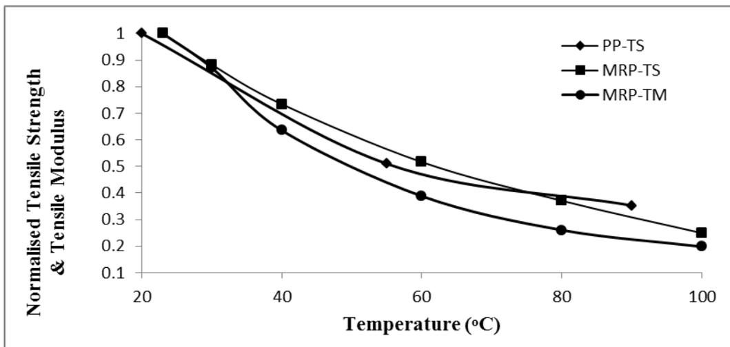
Figure 6. Comparison of different thermoplastic at elevated temperature
