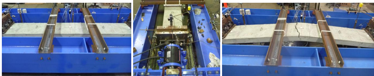
(a) Test setup: side view (b) Details of connections (c) Buckling failure Figure 1. Long-term test set-up and representative buckling failure mode
