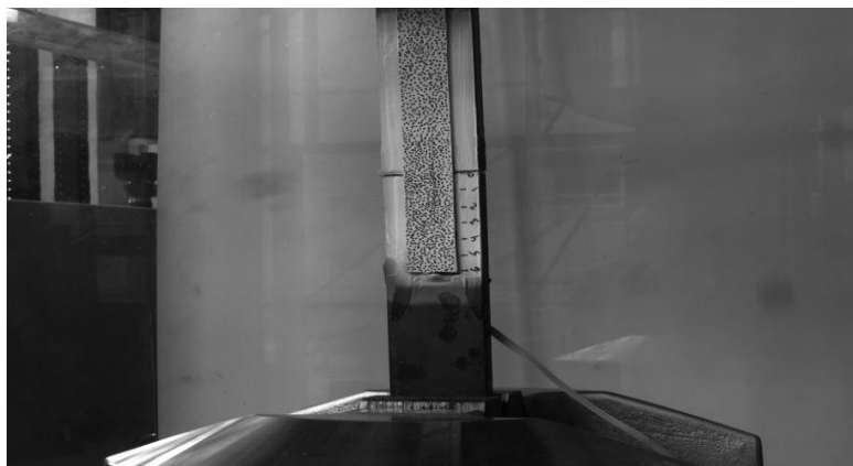
Figure 1. CFRP-steel double-strap specimen under static loading showing the face with VIC-3D camera strain capture
