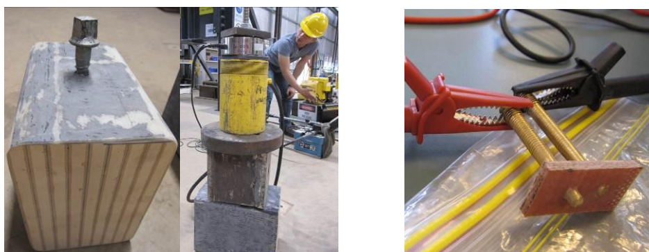
Figure 3. Pulling strength test of screw spike (left) and direct-current insulation resistance (right)
