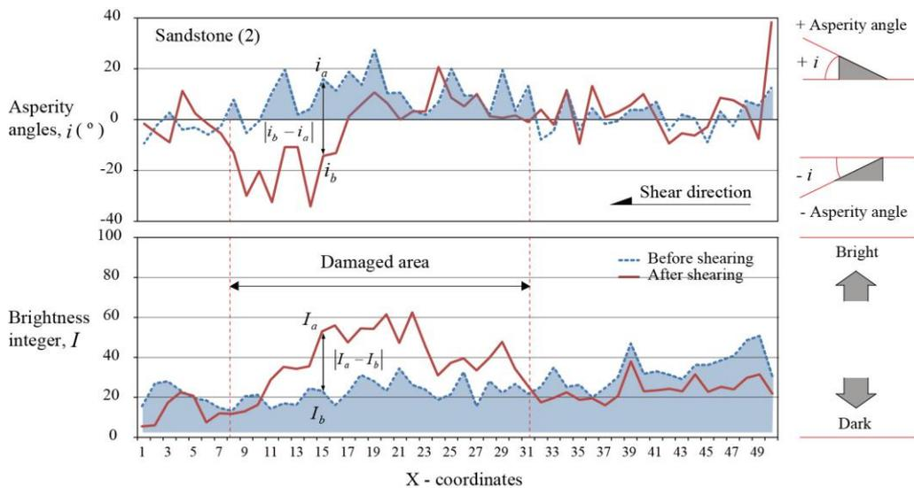
Figure 5. Brightness integers of greyscale images and asperity angles, sandstone (2)
