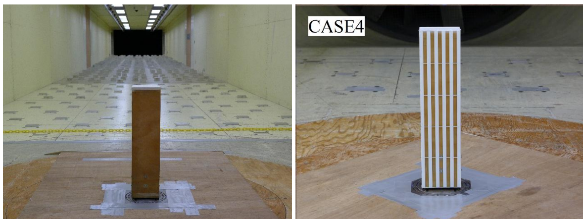
Figure 2. Test building model with a double-skin facade in HKUST's boundary layer wind tunnel
