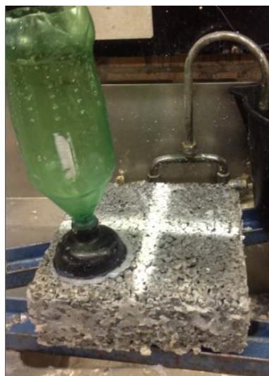
Figure 2. Infiltration test set-up on pervious concrete specimens
