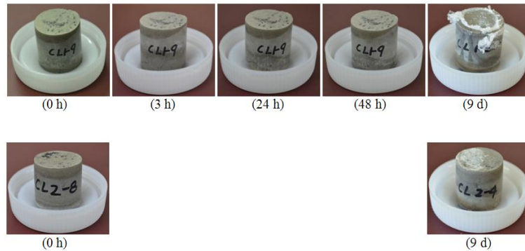
Figure 4. Changes of appearances of geopolymers GPC-Na 2 O · 1.5SiO 2 (CL1) and GPC-NaOH (CL2) under water contact conditions
