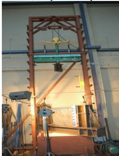
(b) Specimen in impact drop rig
